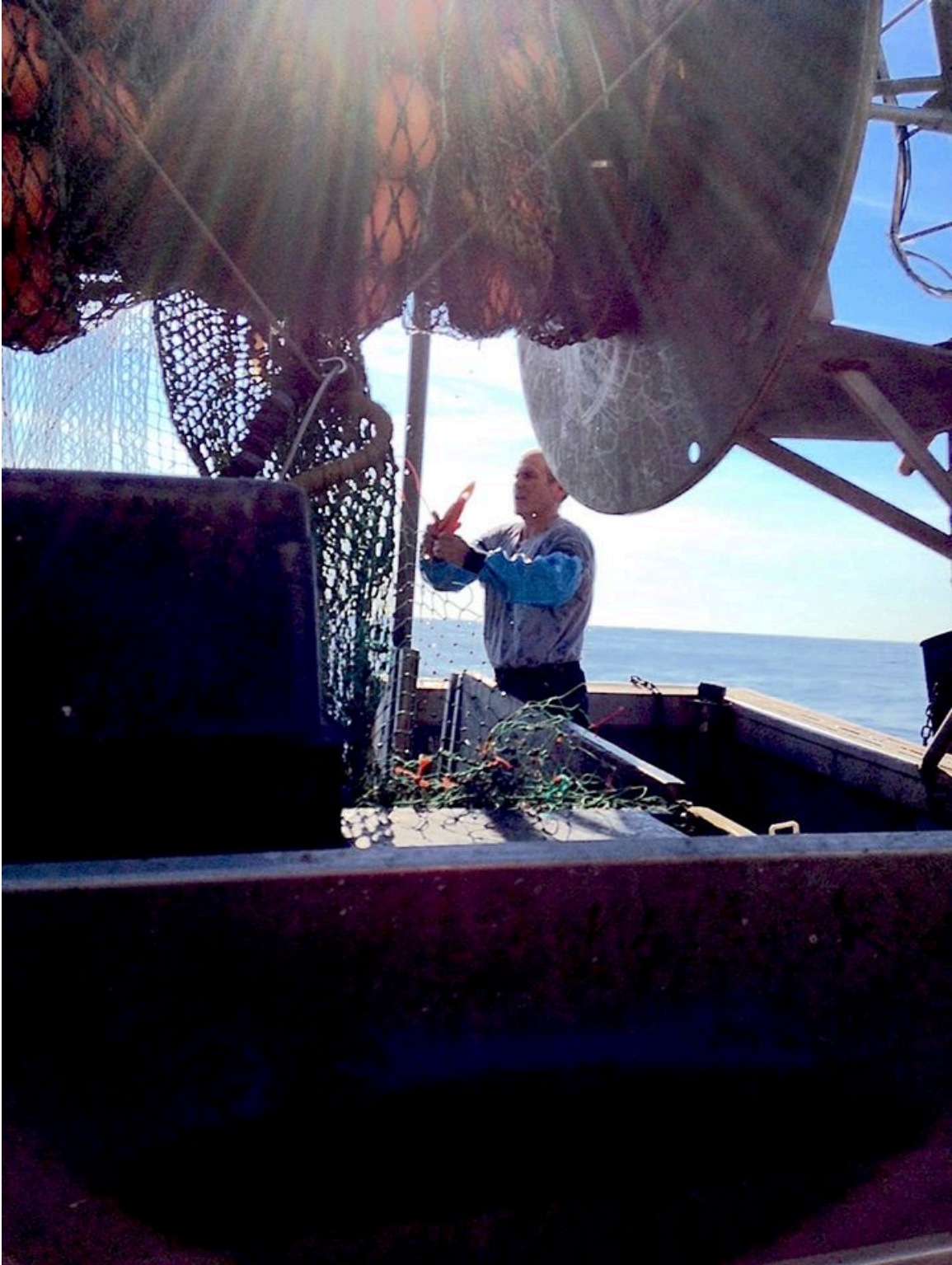
Photo 2. Captain Steve Arnold installing large mesh belly panel into net on F/V Elizabeth Katherine
