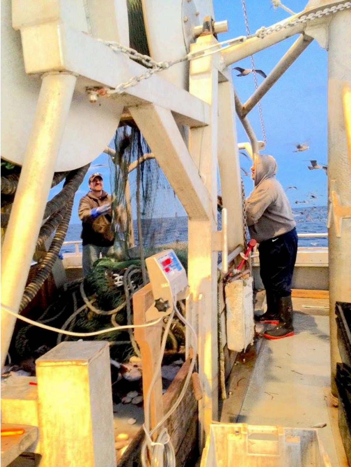
Photo 8. Removing cover from large mesh belly panel in the experimental net aboard F/V Sea Breeze Too
