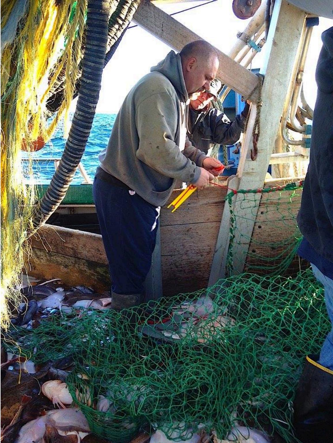
Photo 7. Crew member aboard F/V Sea Breeze Too sewing cover over large mesh belly panel in the experimental net
